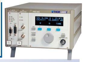
The PDA8000 is designed as a plug-in module for the PRO8000 chassis detailed on page 364. The module is recognized by the chassis when powered. All of the control functions of the photo-current amplifier can be used in manual or remote modes.
